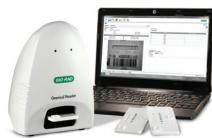
Geenius HIV 1/2 Supplemental Assay differentiates antibodies to HIV Types 1 and 2 in whole blood, serum and plasma. Following a three-step procedure, the cassette is read by an automated reader with band interpretation by validated software.
